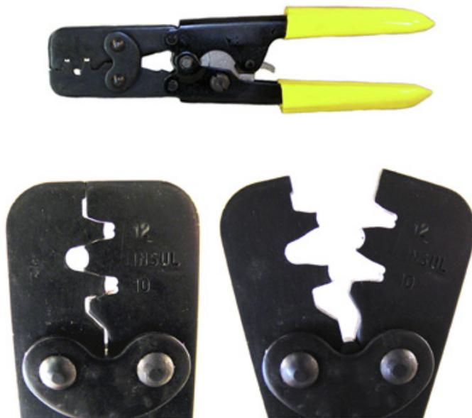
**T-17 Seal and Open Barrel Terminal Crimper**
