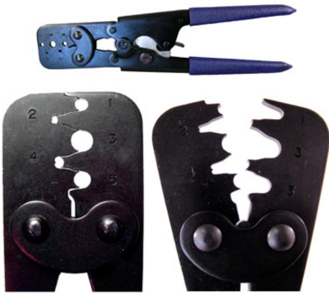
**T-13 Seal and Open Barrel Terminal Crimper**
