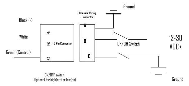
When using the 2<sup>nd</sup> Switch, the light will dim to 75% power. Turning the switch off will toggle back to full power. This is to be used when your vehicles charging system cannot produce the necessary voltage (13.5V or higher) to keep the vehicle charging. Included with your light is an inline "Hi-Low" adapter in case you **DD NOT** want to wire a secondary "On/Off" switch.
