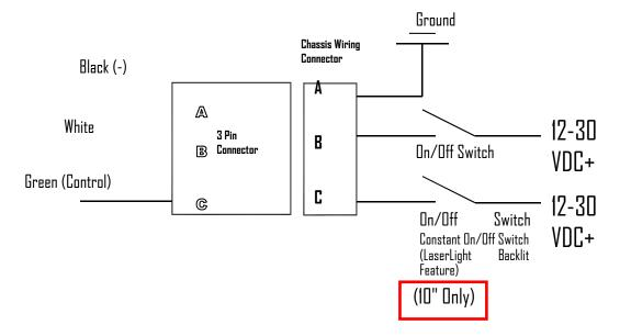
When using the optional second switch, depressing the switch will turn on the Laser section/backlit feature. Depressing the switch again will turn the backlit light off.
